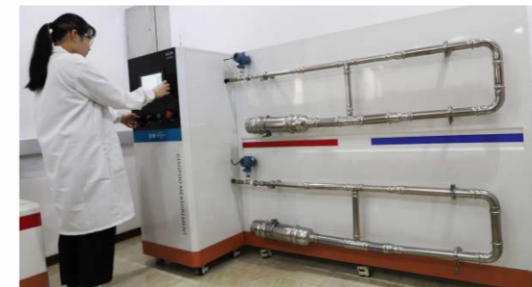
负压试验 Negative pressure test
